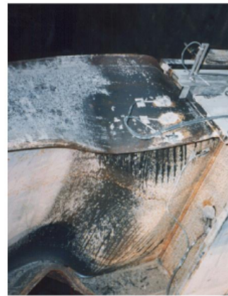
Figure 3: Yielding and buckling pattern of prototype SidePlate™ Uniaxial Test Specimen 3.
