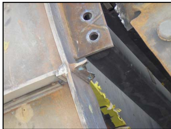
FIGURE 14 BRITTLE FRACTURE OUTLINE AND LOCATION IN BEAM’S BOTTOM FLANGE, PREDICTION VS. TEST FOR THE ‘TRADITIONAL’ CONNECTION TEST ARTICLE.
